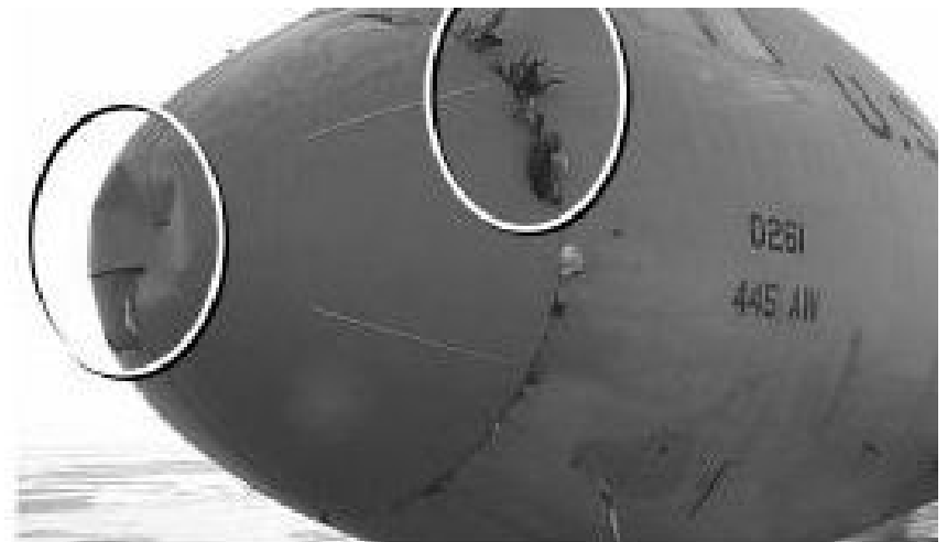
Cargo 141 damage and bird remains from collision with a Canada goose.
